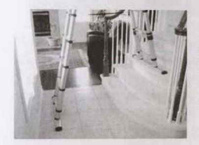
4. This will stop and lock the Combi- ladder at this position and it will now be ready to be used on the stairs as shown in FIGURE 9
